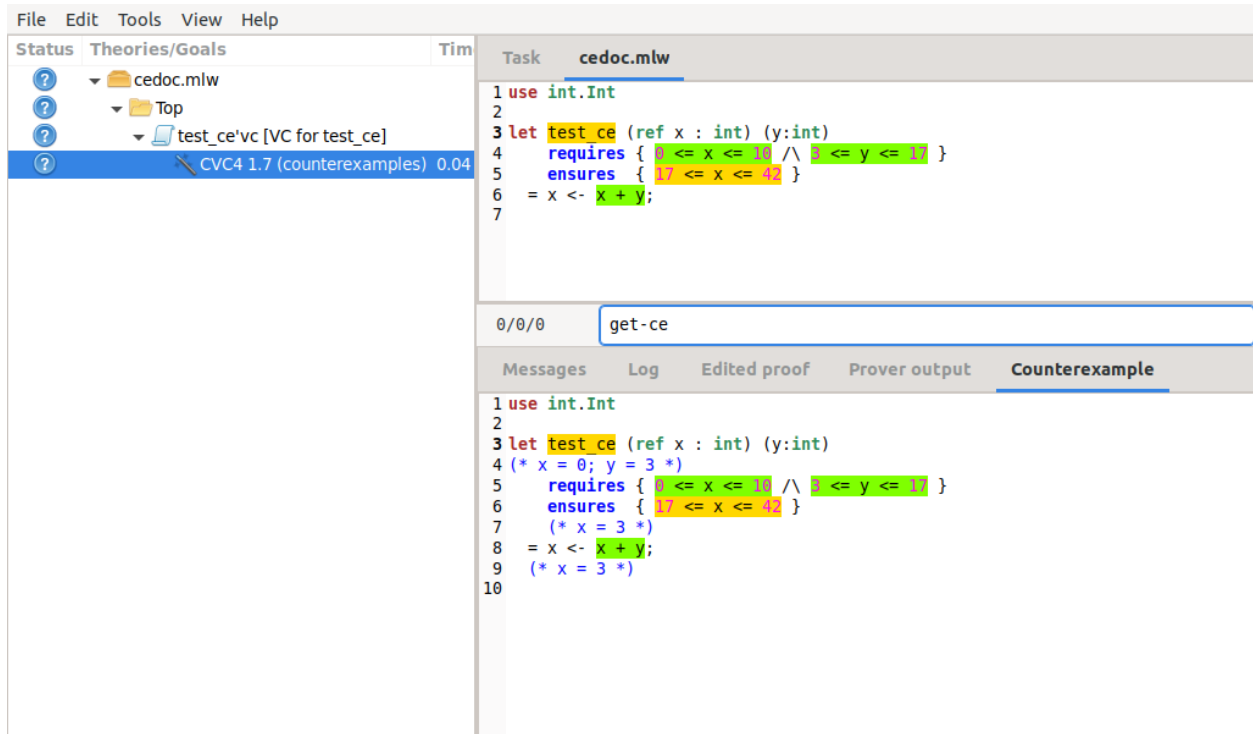
Fig. 6.2: Counterexamples display for CVC4
